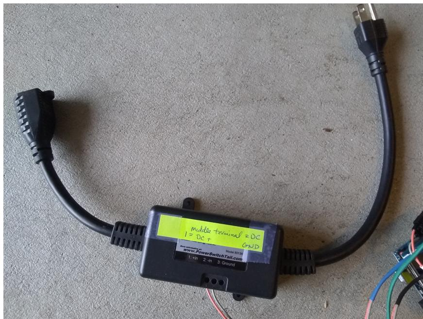
Figure 3: Relay controlled power pass through - PowerTail II
