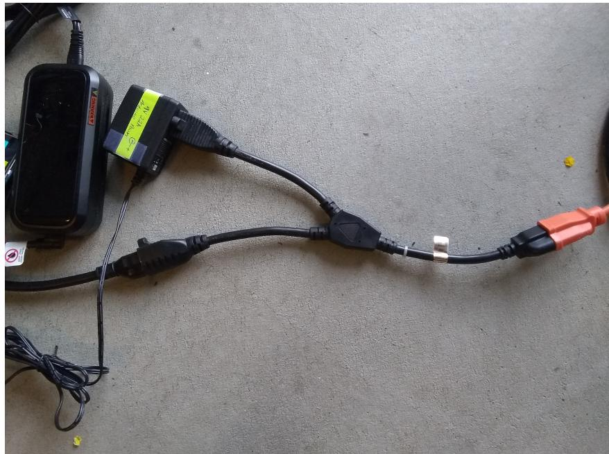
Figure 4: A Y-splitter for providing power to the Arduino and charger
