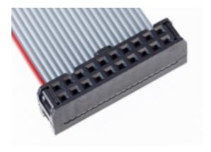
Then add crimped on ribbon cable female sockets to the cables and push onto male pin headers on your strip board. Mount your serial connectors for programming, switches, push buttons, leds, and battery holders, battery chargers and voltage regulators, sensors and controllers to the strip board, and start programming. I'll bet you will be proud of your results.
