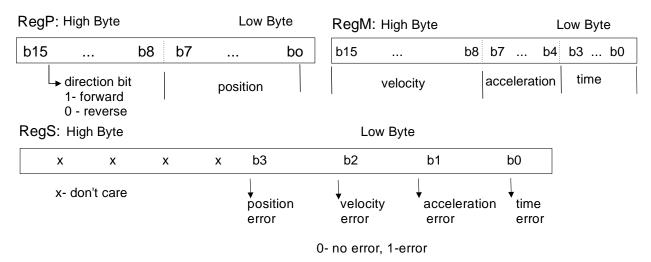
**Position, velocity, acceleration, and time** define a **motion.** RegS indicates **errors**.
